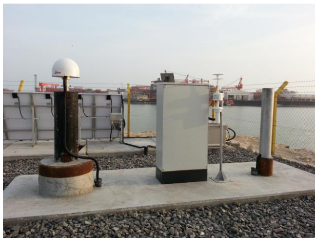
A completed borehole station on one of the manmade islands in the Caspian Sea
