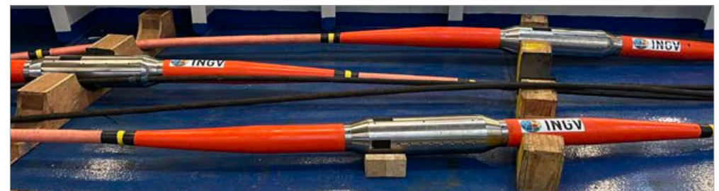
Image 6: The three instrument pods on laid out on the cable-laying deck awaiting deployment
