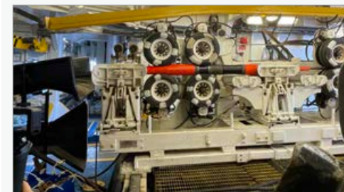
Image 12 (Top): The seven universal joints required to splice the repeaters into the cable. Image 13 (Bottom): A universal joint passing through the cable engine on the cable deck.
