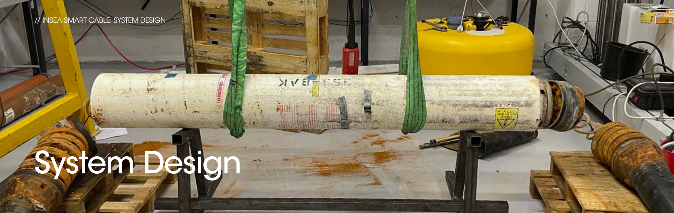
Image 4: One of the three decommissioned repeater housings prior to being reconditioned and retrofitted with the seismic instrumentation.
