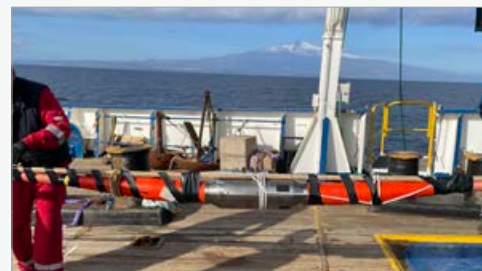
Image 16 (Top): Repeater being deployed Image 17 (Bottom): Instrument pod being deployed
