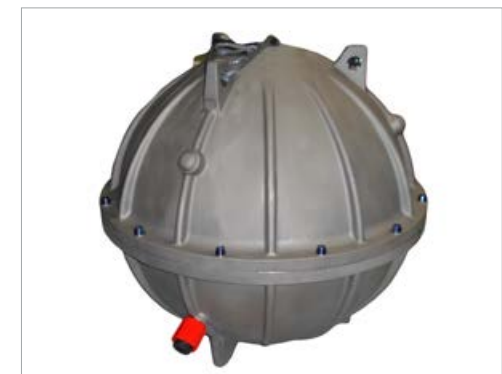
Image 1: The observatory grade cabled Orcus OBS is designed to be placed on the seafloor.
