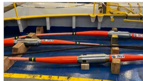
Image 10 (Top): Two of the repeaters on the deck of the Antonio Meucci Image 11 (Bottom): The instrument pods on the cable-laying deck of the Antonio Meucci
