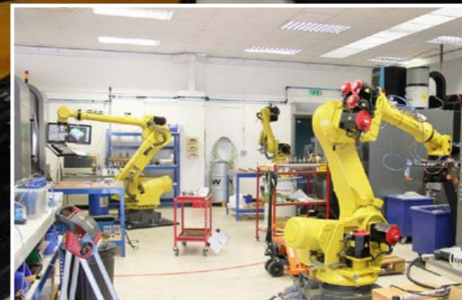
INCLUDED WITHIN OUR CNC MACHINING CAPABILITY ARE THREE ROBOTICALLY TENDED 5-AXIS MACHINES AND A WIRE ELECTRICAL DISCHARGE MACHINE.
